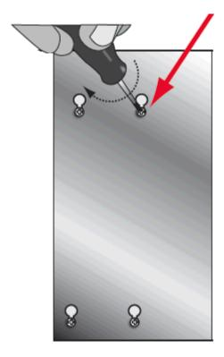
c. Inside the cabinet, screw in the two self-tapping screws (supplied in the product box) at the top and bottom of the power supply.
